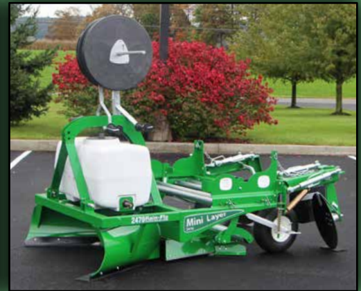
Water Tank for Weight
