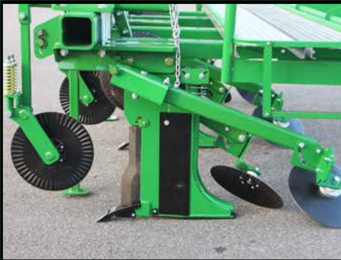
Built with Replaceable Wear Points
