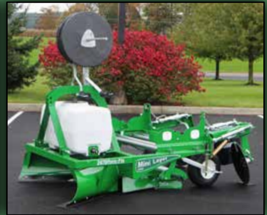
Water Tank for Weight
