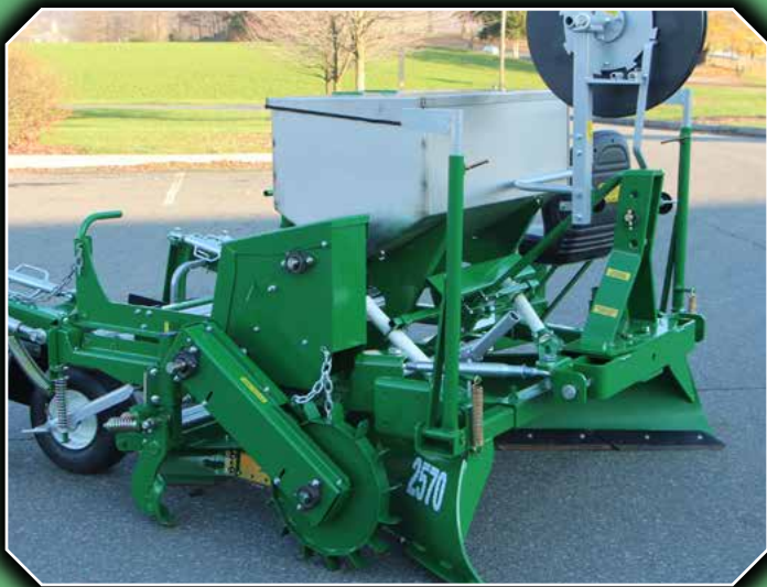
Drive Wheel and Gear Box
